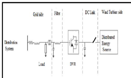
Fig. 1 Complete Configuration of the proposed inverter with FACTS capability.
