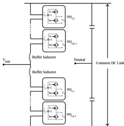
**Figure.2. Structure of a Single Phase MMC Inverter**
