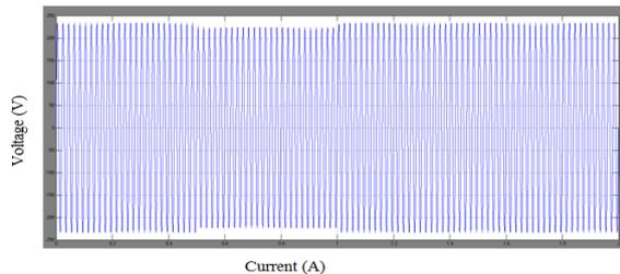
**Fig. 8 Output waveform without DVR**
