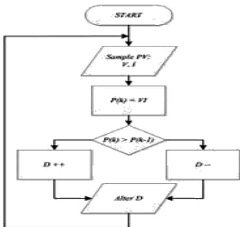
**Fig.3. Flowchart for hill climbing technique operating voltage of the DC link between the array and the power converter**
